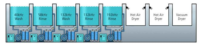
Drying stations, automation, and environmental enclosures can be added as needed. Class 10 or 100 cleanroom on site.
